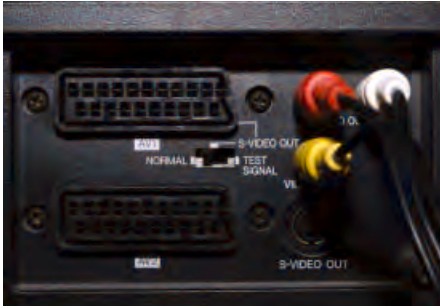
Here the connection is set up for composite video and stereo audio, but the S-video socket below would provide a better-quality connection
